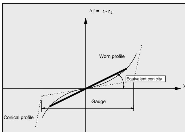
Figure 4: Equivalent conicity
