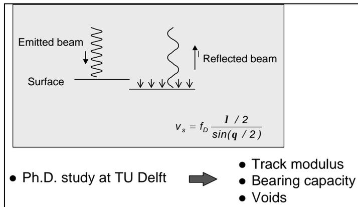
Figure 3: HSD (High Speed Deflectograph)
