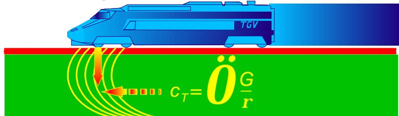
Wave propagation dependent on vertical track stiffness
