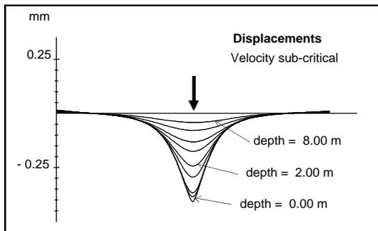
Figure 6.b. Displacements under subsonic steady state load
