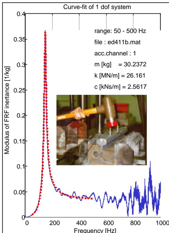
Figure 9 FRF of a 0.5 m sample of ERS
