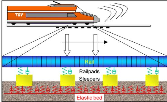
Figure 6 Modelling of vehicle and track structure in RAIL
