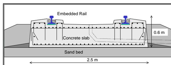
Figure 8 Schematic cross-section and detail of ERS
