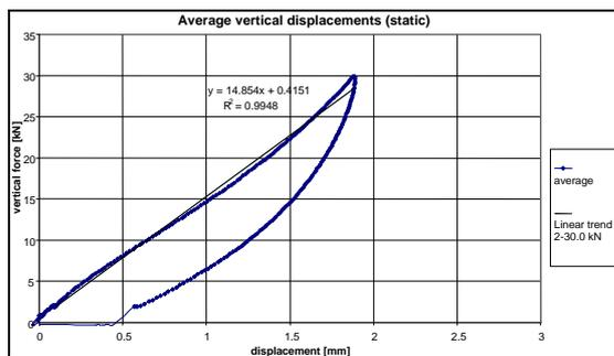
Figure 3 Typical load-displacement diagram of track structure
