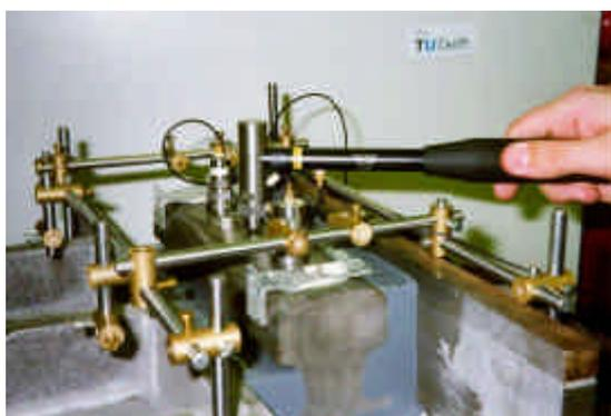
Figure 4 Hammer excitation test on an experimental Embedded Rail Structure
