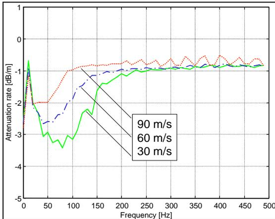
Figure 14 Attenuation rate of optimum designs (multicriteria optimization)
