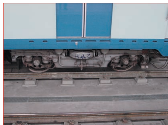
Fig 4. Edilon Block System
