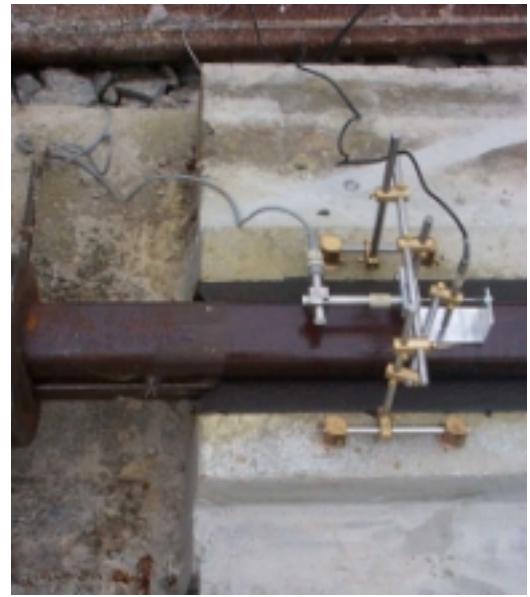
Fig. 3.5.1: Tests on the longitudinal elasticity of the new embedded rail structure.
