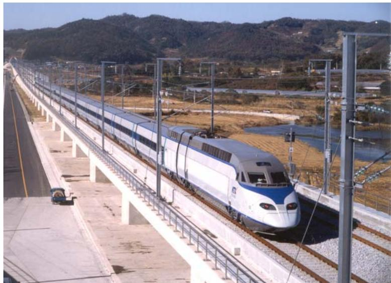
*Figure 1 Ballasted high-speed track (Korea)*
