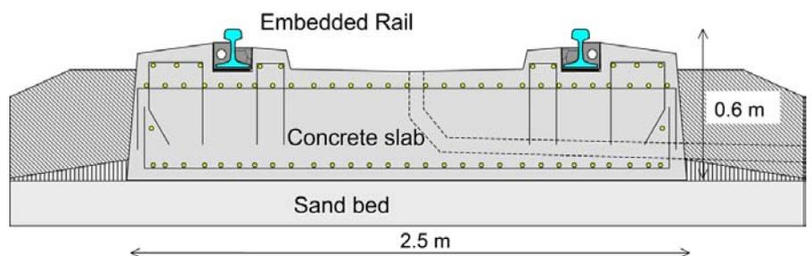
Figure 6 Embedded rail track near Best (NL)
