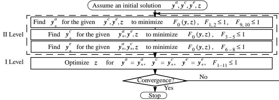
Figure 3. Flowchart for two-level optimization of the truck
