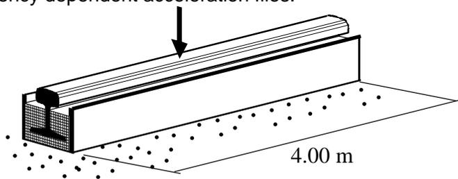
Instrumented hammer test
