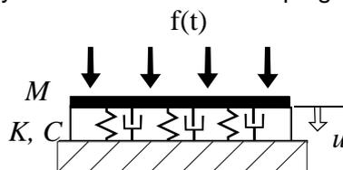
Stiffness, damping and mass properties of the elastic bed
