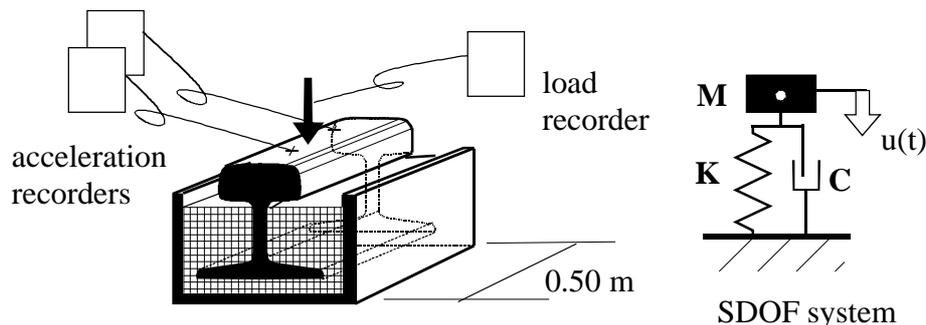
figure 6 instrumented hammer test
