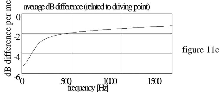
The distance damping shows us much damping of the low frequencies and a much smaller damping of the high frequencies. Because of the limitations of the model the shape of this result could be expected.
