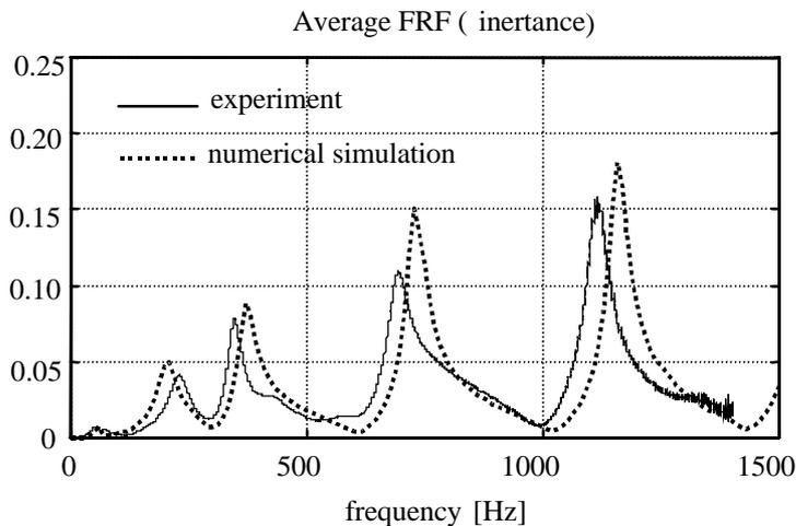
figure 10 FRF of a 4.00 m specimen
