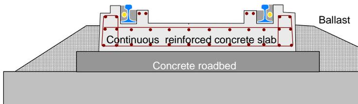
**Figure 2 Embedded rail construction**
