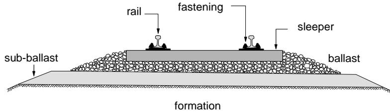
**Figure 1 Construction principle of classical track structure**
