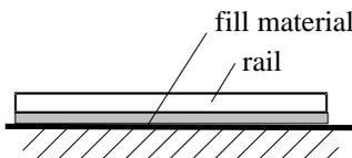
**Figure 4 Model of embedded rail on rigid foundation**
