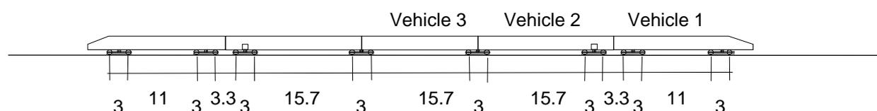
Fig. 1: Model of the Thalys (dimensions in m)
