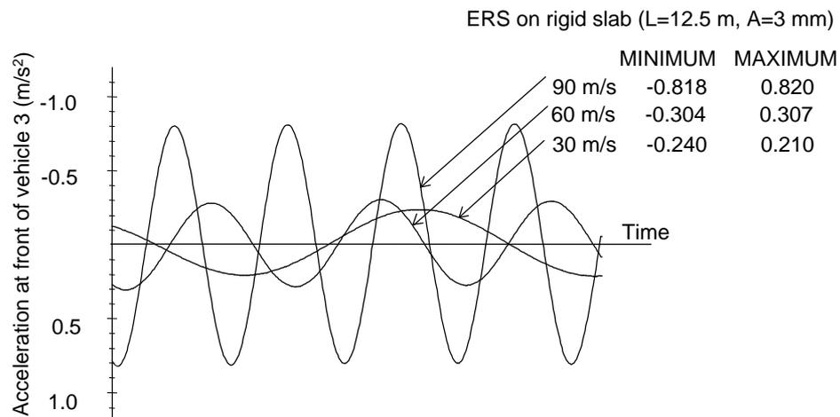
*Fig. 7: Acceleration at front of vehicle 3*
