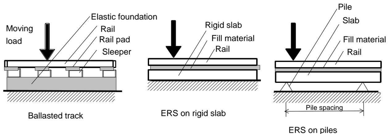
Fig. 3: Track structures used in the analyses
