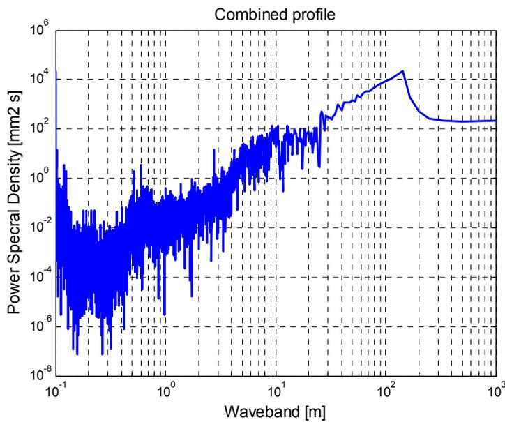
Figure 10 Total vertical geometry versus frequency (PSD function)
