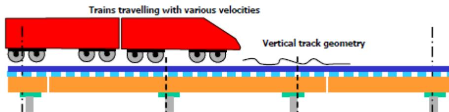
Figure 9 Schematic representation of the FE model used in the dynamic analysis
