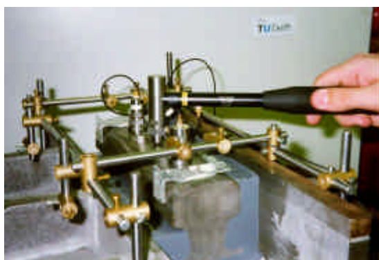
Figure 4 Hammer excitation test on an experimental Embedded Rail Structure
