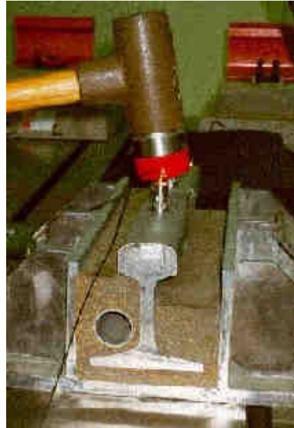
Hammer excitation testing of embedded rail construction
