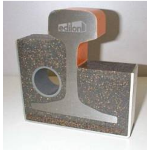
The present design of embedded rail was modeled and several types of loading were simulated.
