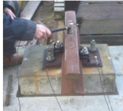
Fig. 3: Single rail fastening assembly RET on a block
