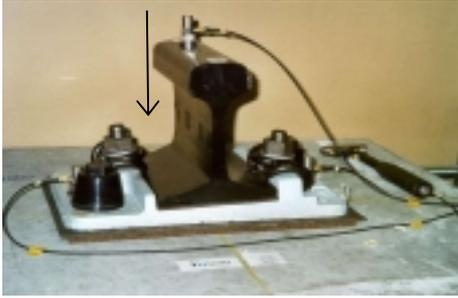
Fig. 1: Single rail fastening assembly HSL tested in laboratory
