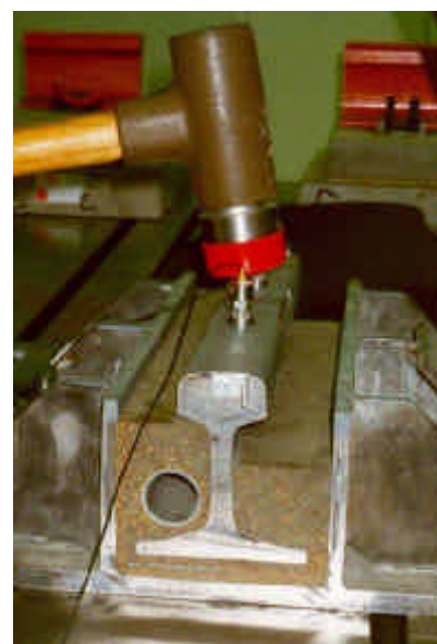
Figure 2. Hammer excitation testing of embedded rail construction
