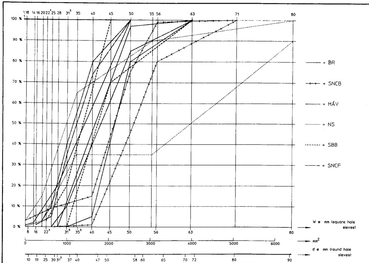
Fig. 1: Examples of ballast grading used by railways
