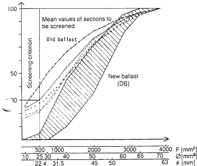
Fig. 4: Summary of old ballast analysis for DB sections
