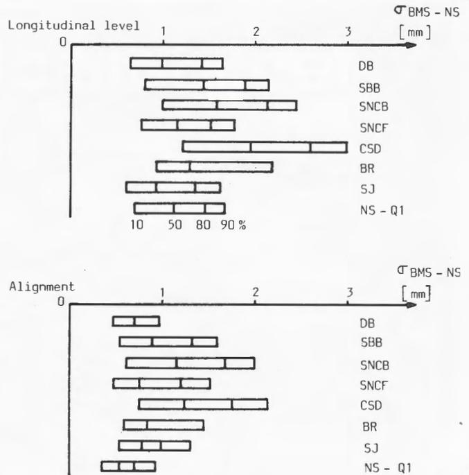
Fig. 6: Standard deviation distributions of level and alignment measured by BMS on several European networks
