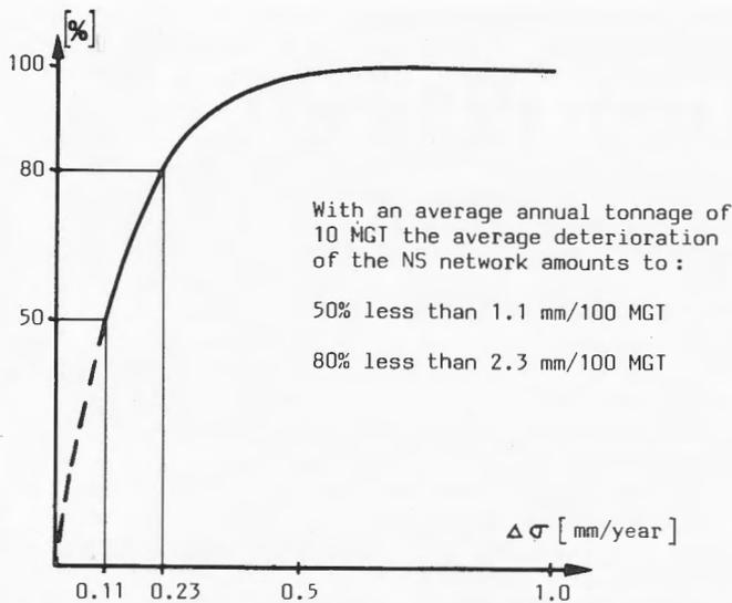
Fig. 5: Distribution of track deterioration on NS for 600 MAINS. (3500 km of track)
