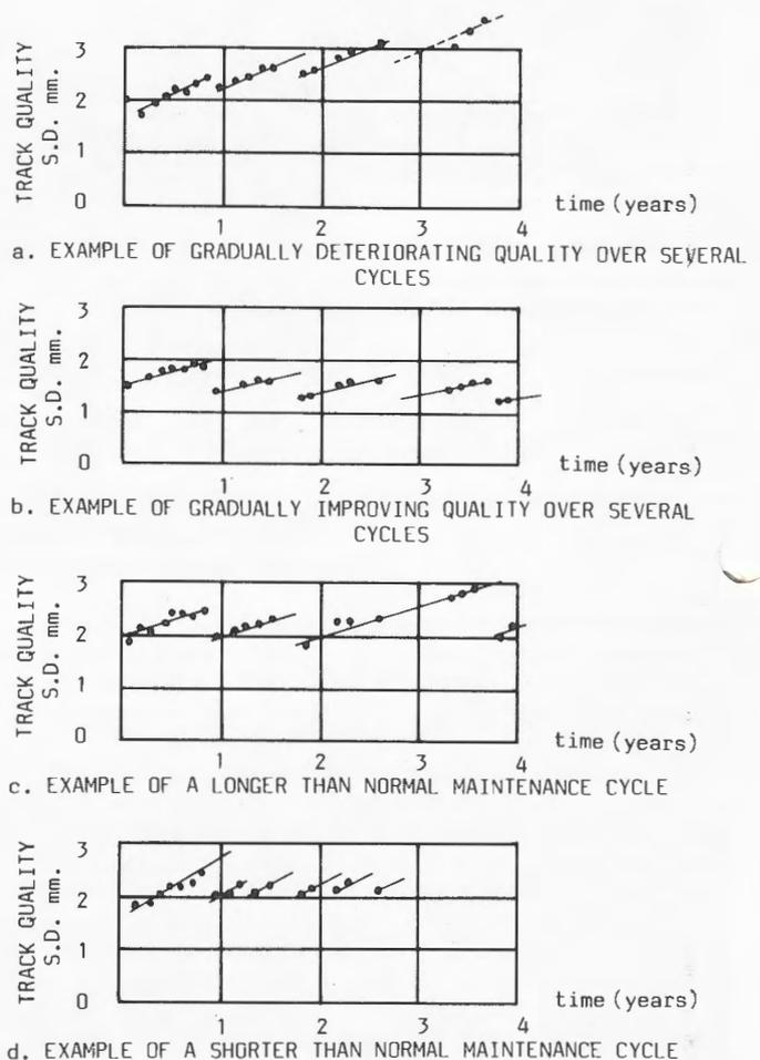
Fig. 7: Various trends of track deterioration observed on BR test sections
