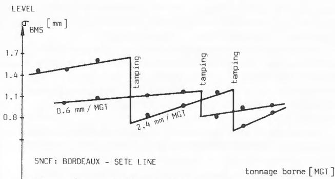
Fig. 8: Deterioration scatter between two close track sections
