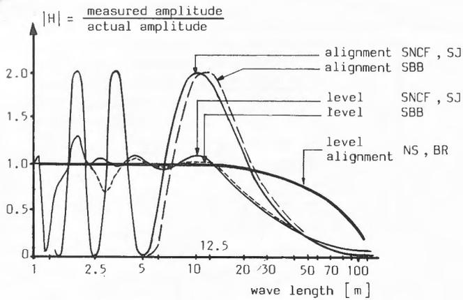
Fig. 2: Transfer functions of various recording cars
