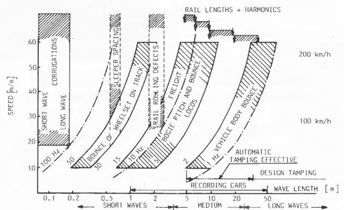
Fig. 1: Relevant wavelengths in vertical geometry
