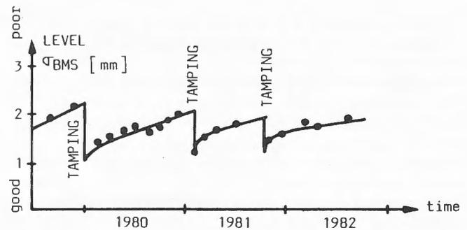
Fig. 4: Historic data for track quality on a BR test section
