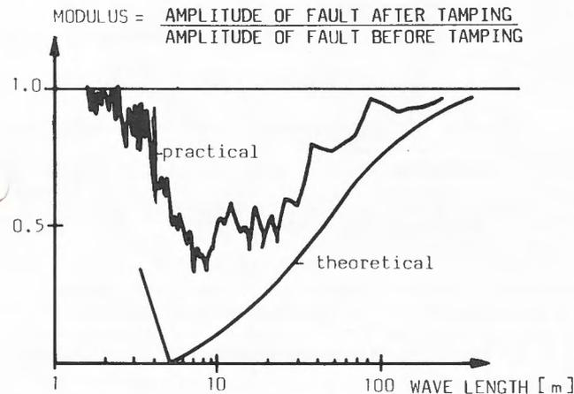
Fig. 3: Transfer function for levelling by a PLASSER 07-16 tamping machine
