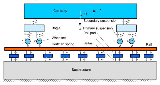
Figure 3.1 A vehicle-track model (a single coach on a classical track) in DARTS\_NL
