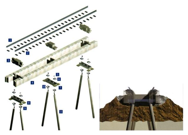
Figure 2.5 Constructional principal of NFF structure
