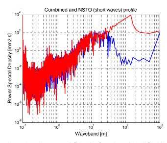
Figure 3.4 Power Spectral Density of measured (blue line) and combined (red line) vertical rail level geometry profiles.
