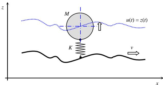
**Fig. 1** Mass-spring system disturbed by rail irregularity
