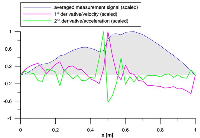
Fig. 3 Non-dimensional weld geometry, first and second derivatives
