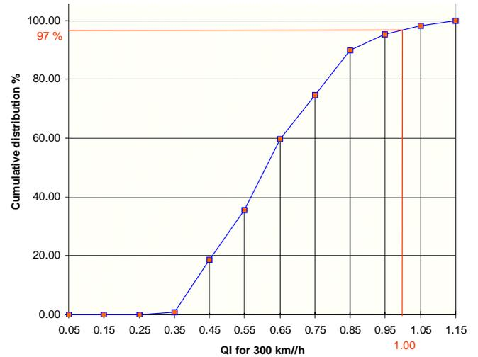
**Fig. 12** Cumulative distribution of QI for vertical rail geometry pertaining to 300 km/h. QI=1 corresponds to a 1<sup>st</sup> derivative of 0.7 mrad.
