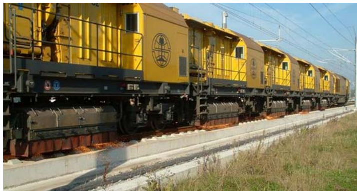
Figure 15 The Speno grinding train on the HSL-South
